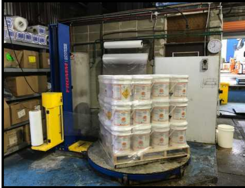
BLENDING PLANT AUTOMATIC STRETCH WRAPPING MACHINE
