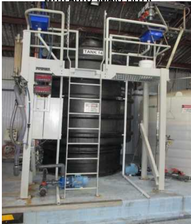
10,000L FIBREGLASS MIX TANKS SUITABLE FOR ACIDS/CHLORINE BASED SPECIALITY CHEMICALS WITH AUTO SMART FILLER
