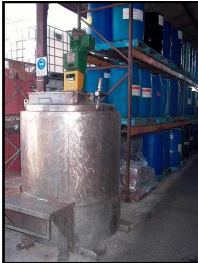
1200L FLAMMABLE HEATED MIXING TANK
